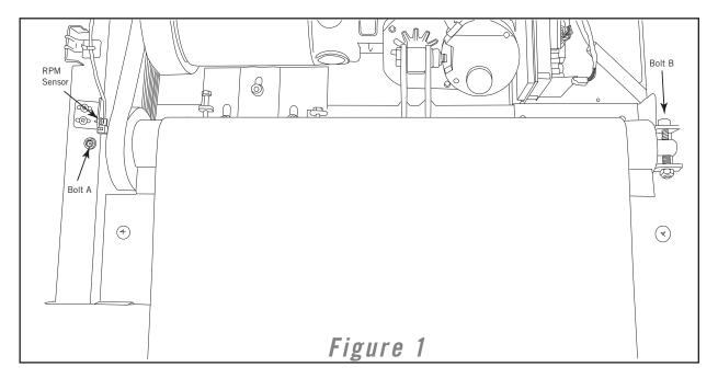
3) Detach tension bolts and remove the rear roller.
