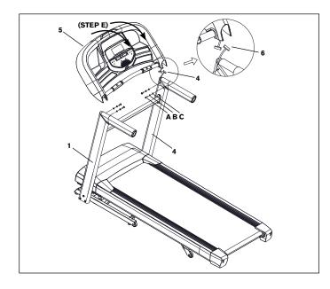
NOTE: Be careful not to pinch any wires while assembling the console.
