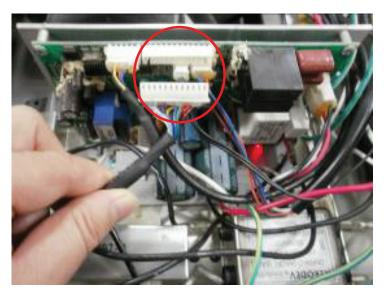
b. If output is around 15VDC, check the console cable for pinches or kinks. If any damage is found, replace the console cable. Disconnect the console cable at the UCB and measure the DC voltage between the "GND pin" (Pins 4 & 5) and the "+ 15V Pin" (Pins 7 & 8). DC output is normally around 15VDC. If there is no output, replace the console cable.
